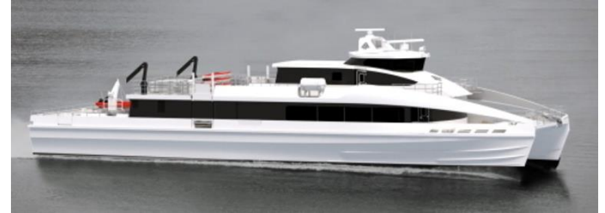
Hybrid vessel for Nordland is extended to carry the weight of batteries and fossil fuel. 40.6 m, 130 pax
