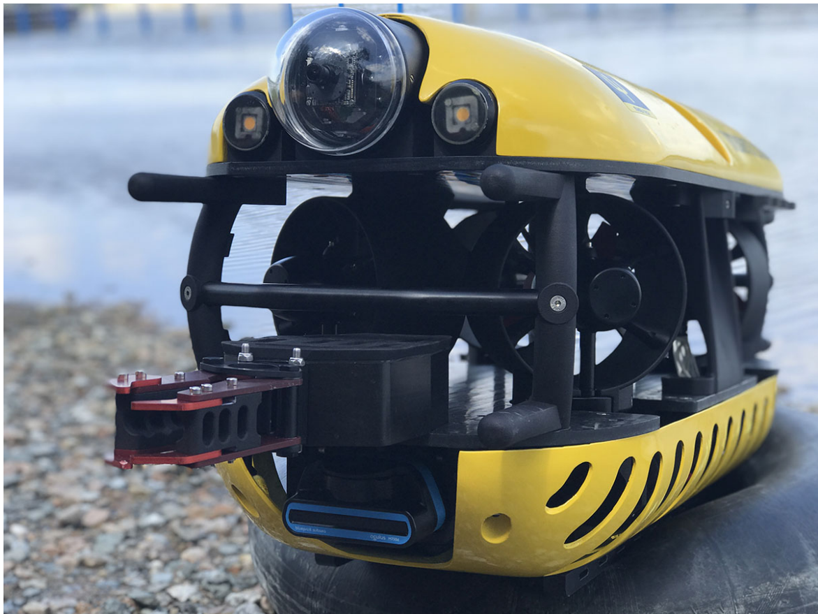
SeaClear’s ROV TORTUGA is known as ‘the cleaner’ robot. It collects the litter from the seafloor. @ SeaClear, 2021
