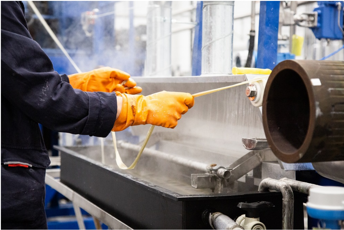
Infinited Fiber wet spinning process. © Infinited Fiber Company, 2023
