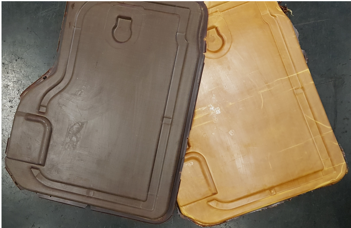
Backseat car panel made from bio-waste. © ECOXY project, 2020
