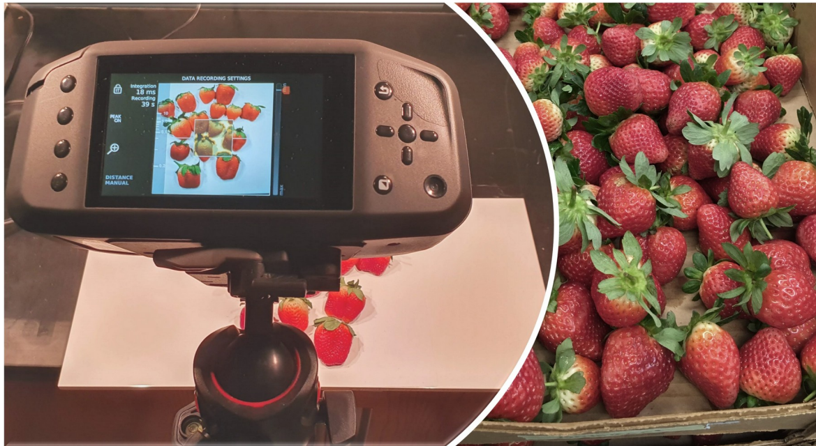
Hyperspectral imaging camera, taking an image of strawberries. © Anastasia Ktenioudaki / FreshProof - 2022
