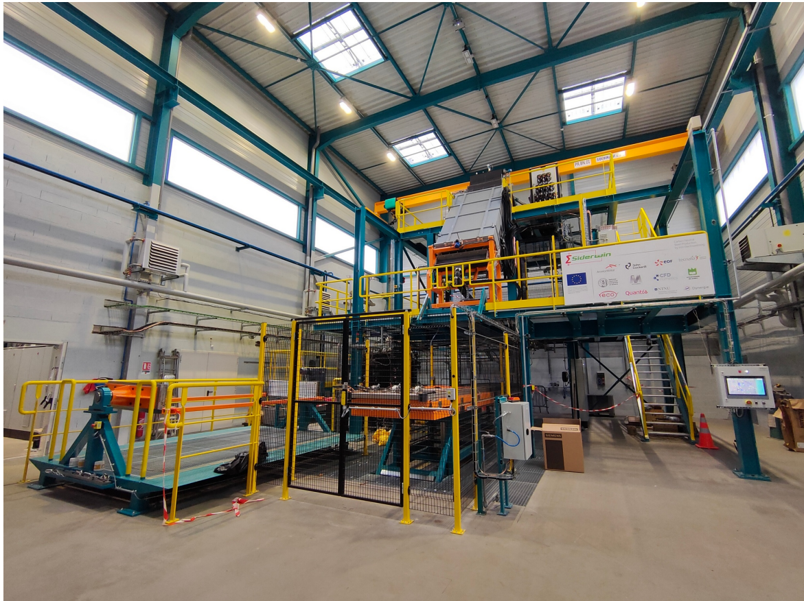
ArcelorMittal's pilot plant in France uses electrolysis to produce iron plates. ©SIDERWIN
